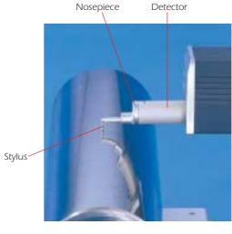
This function determines the coordinate difference between two arbitrary points, such as a step height and a pitch interval.
