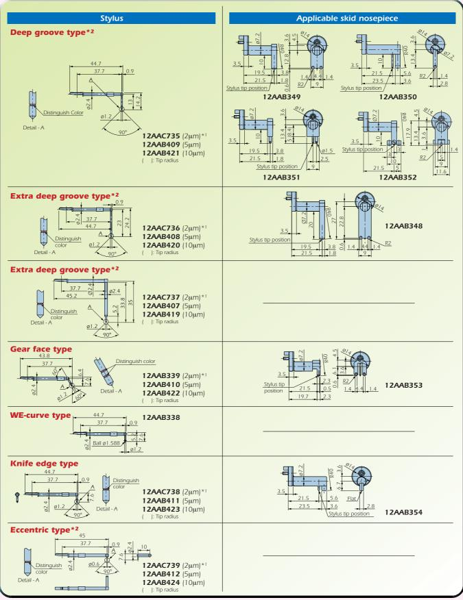
\*1 Tip angle is 60° \*2 At using this stylus, measuring force of the detector does not guarantee.
